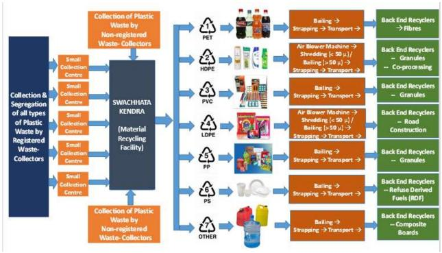
Figure - 4: Systemic Approach for Plastic Waste Collection, Segregation and Recycling
